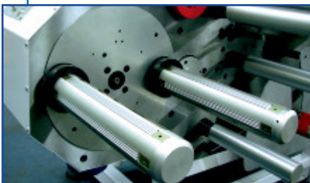
Semi-turret version of rewinders with the option of simultaneous wound on two spindles
